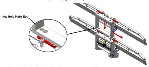
Note: Periodically tighten Security Bolts to ensure secure connection.
